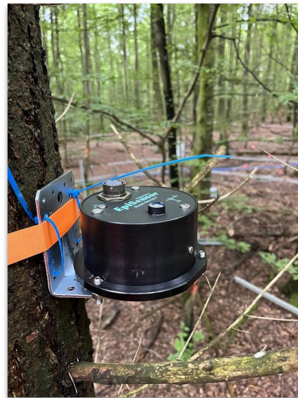
ACCELEROMETER (Episensor - Kinemetrics)
